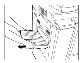
• If a staple sorter is attached, first pull it away from the copier by lifting the release lever.
